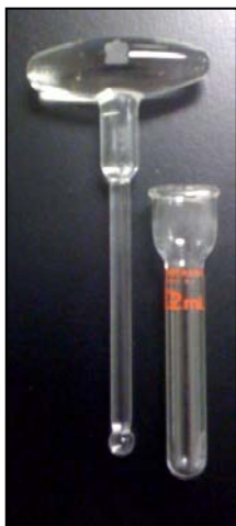
Figure 3 - Dounce Homogenizer. This is a digital image of the dounce homogenizer used for the ChIP assays performed.
