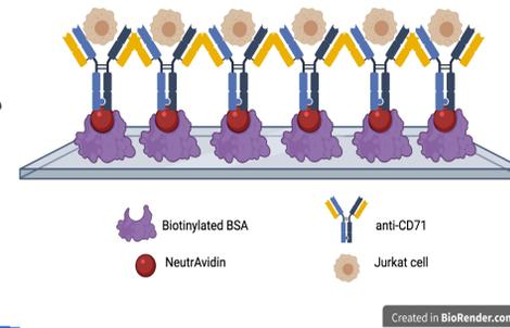
Figure 2B: Antibody ladder to adhere cells to the microfluidic device for observation.
