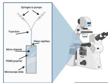
Figure 2A: Anatomy of a microfluidic device attached to an inverted microscope.
