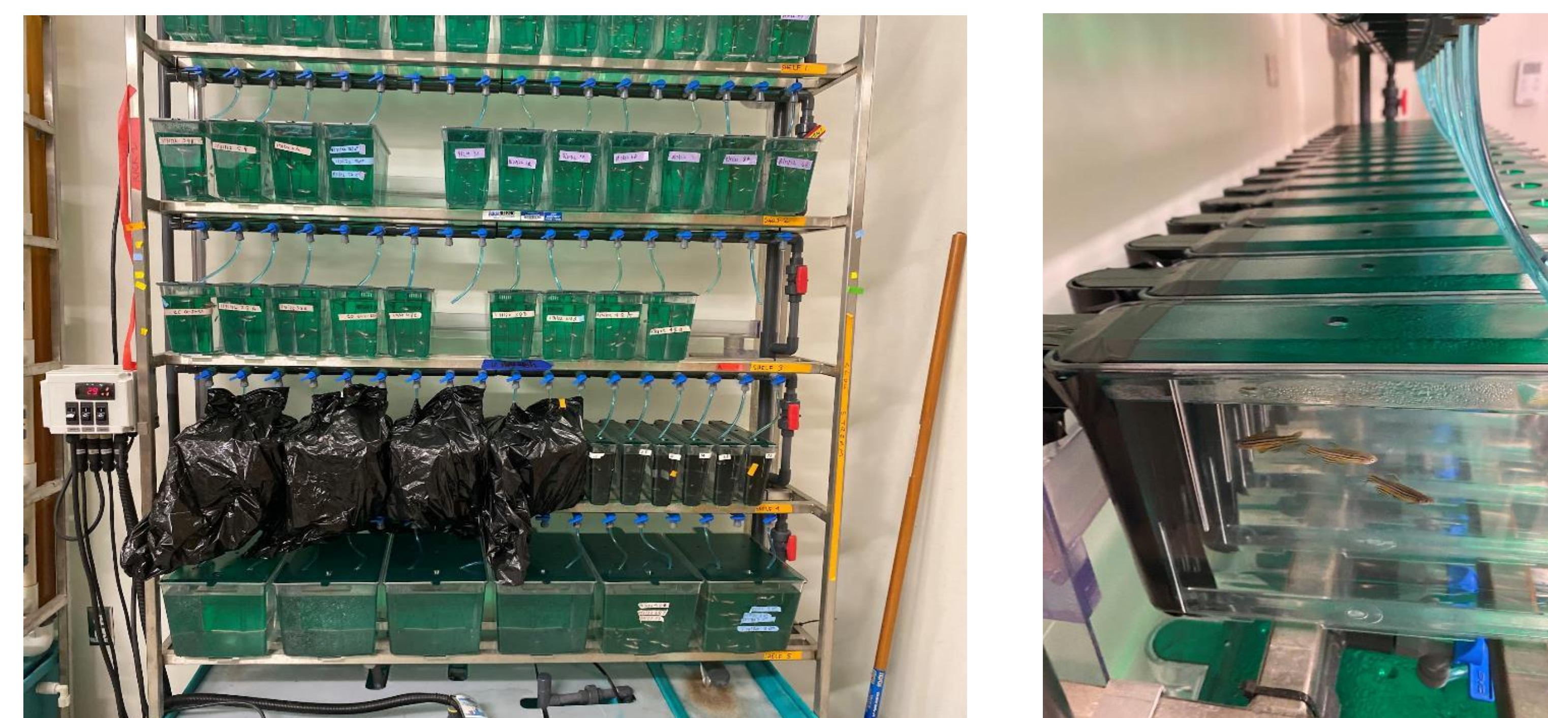
Figure 4. Covering Tanks. Tanks were covered using electrical tape and trash bags. The electrical tape covered the backs of the tanks to prevent exposing fish to light. For the first 14 days, trash bags were removed from all tanks at 7:15 am. The trash bags were replaced at 3:15pm for the short-day group and 7:15pm for the control group. The lights in the lab automatically turned off at 11:15pm. For the last 14 days, time change had to be considered. For the last two weeks, trash bags were removed from the tanks at 6:15 am. The trash bags were replaced at 2:15pm for the short-day group and 6:15pm for the control group. The lights in the lab turned off at 10:15pm.
